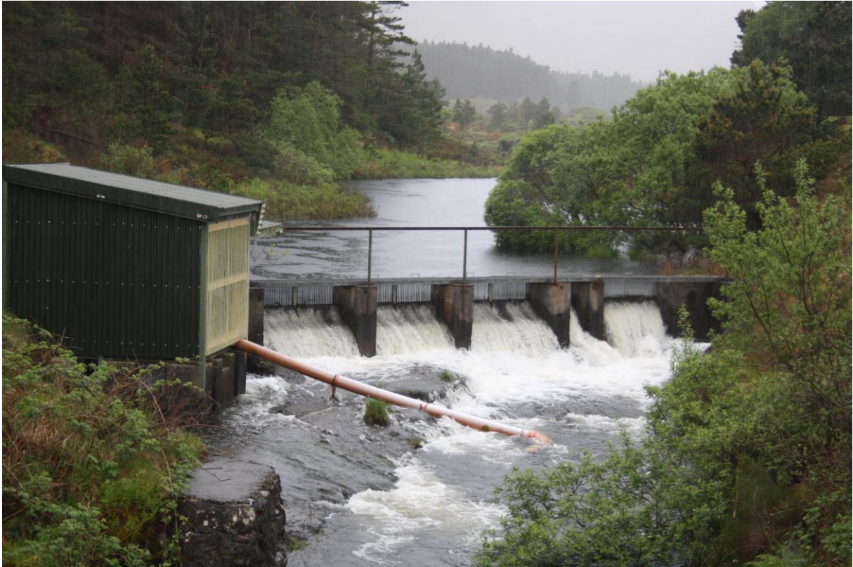
Plate 2 Wolf-trap located along the outflow from Tawnyard Lough captures downstream migrating smolts and kelts. In 2023, this trap was operated daily from March through mid-June. All fish entering the trap were visually classified as salmon or sea trout (kelt or smolt) and a subsample were measured and PIT or acoustically tagged (section 4.2.2 & 4.2.3)
