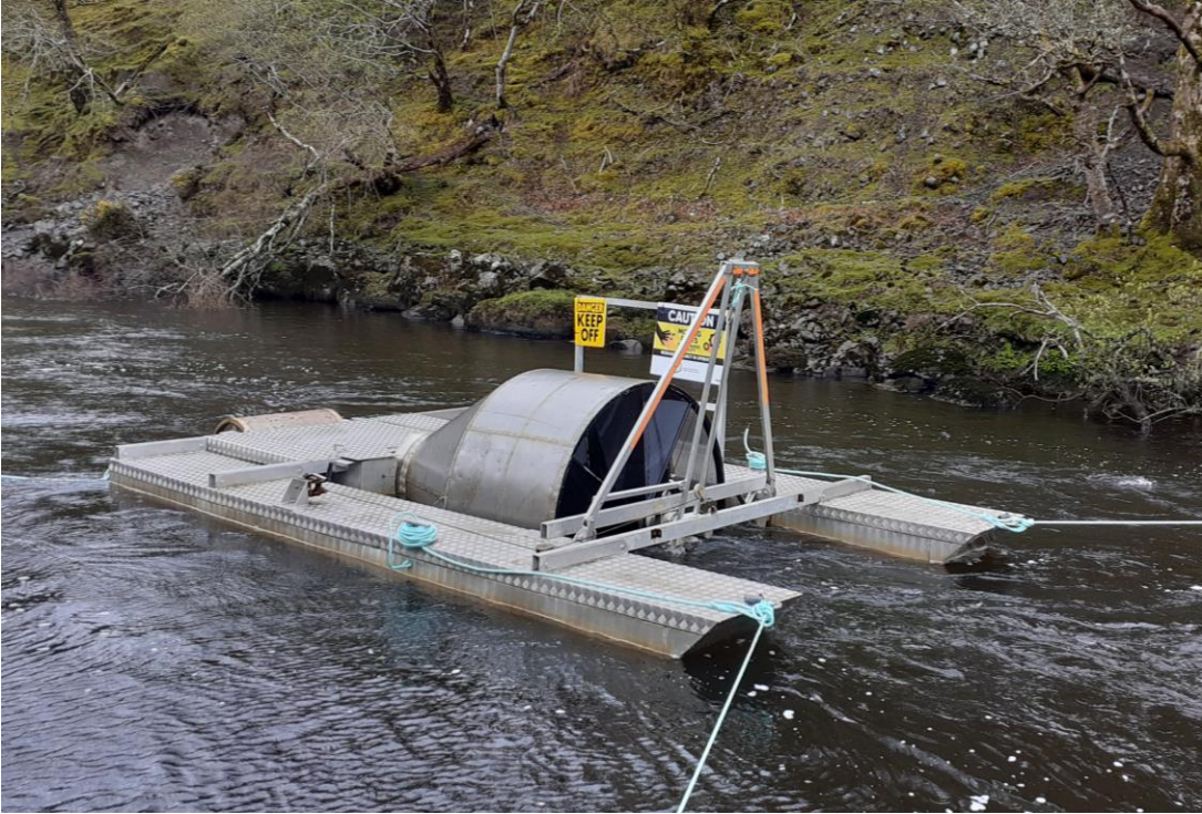
Plate 3 Rotary screw trap for capturing smolts in operation on the main river channel at Erriff Bridge. This trap was deployed during April-May in 2023 primarily for the purposes of capturing emigrating salmon and sea trout smolts for PIT and DST tagging (section 4.2.3)
