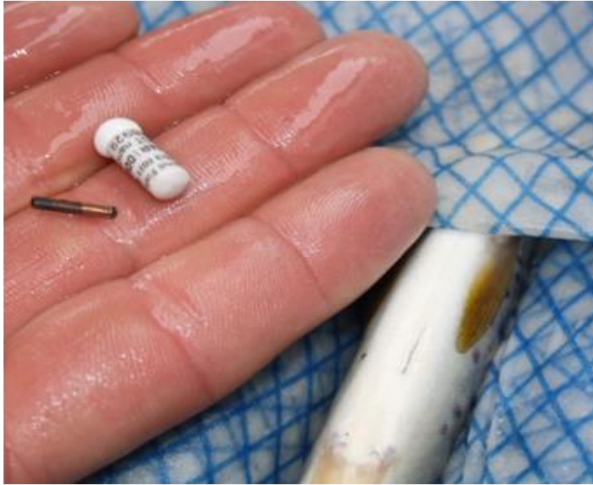
Plate 5 Pit tag and DST tag inserted into sea trout smolt captured at Tawnyard downstream trap.
