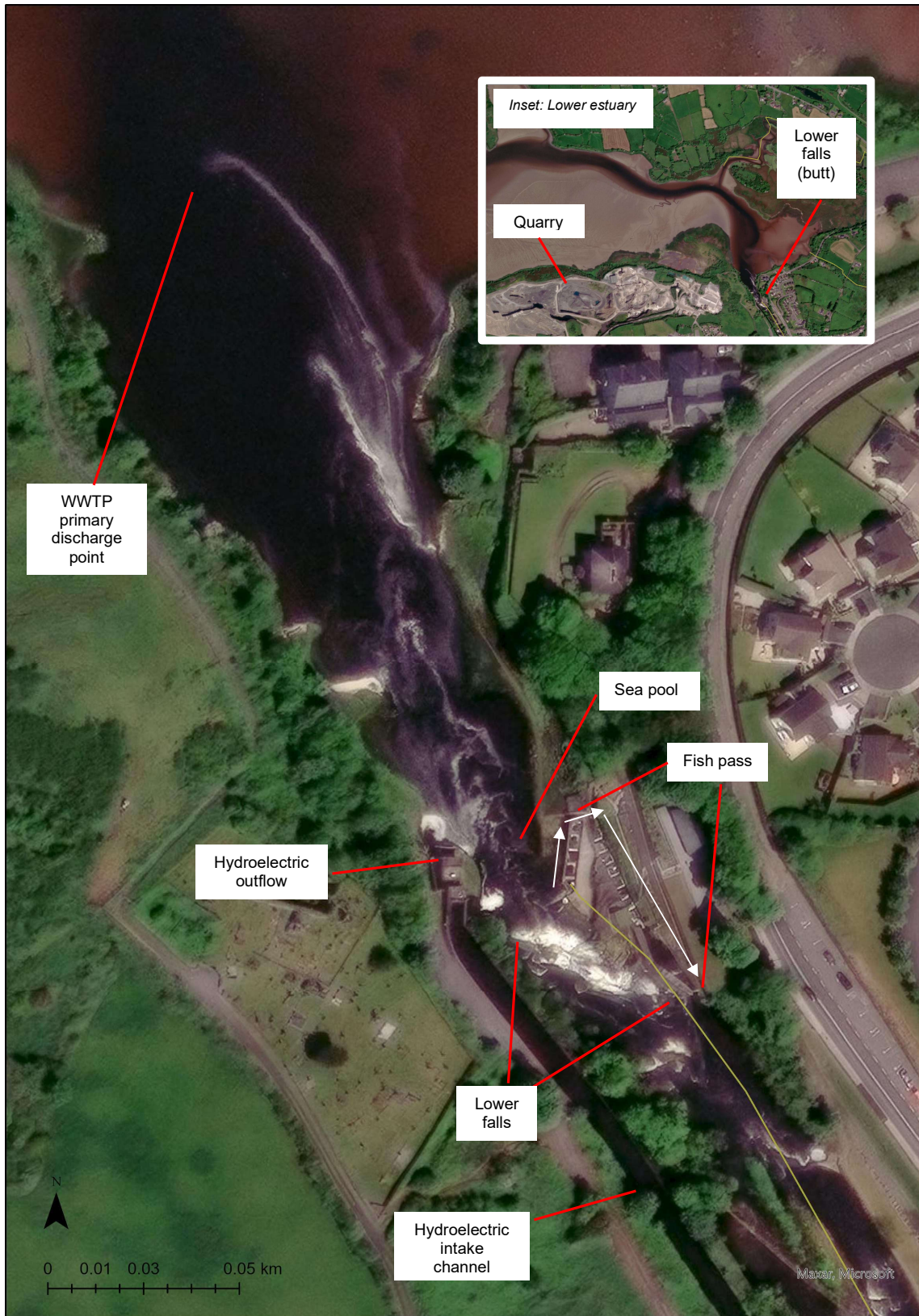
Figure 3a Satellite view of section of Lower Ballisodare from river mouth to immediately above the lower falls (WWTP = wastewater treatment plant). Inset image shows inner estuary and location of quarry (Source: Esri, Maxar, Earthstar Geographics, and the GIS User Community).
