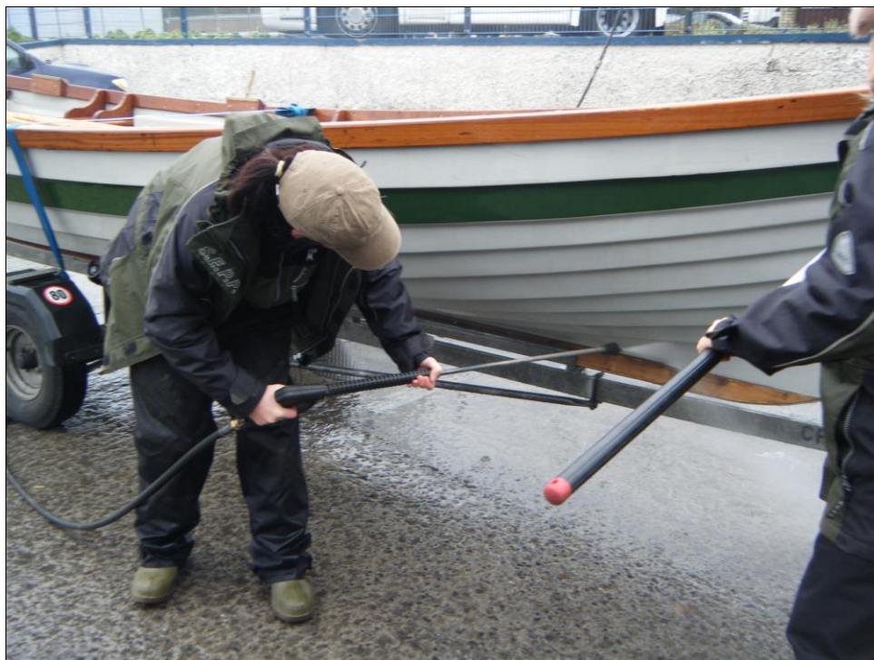
Plate 3.13. Disinfection procedure (steam washing) of a boat being moved between water bodies
