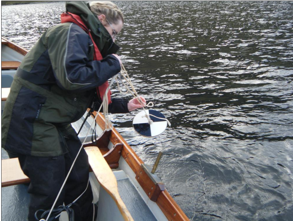
Plate 3.3. Recording secchi depth on Doo Lough, Co. Mayo
