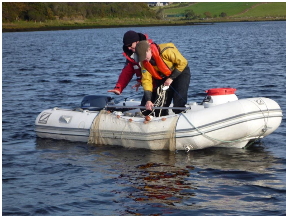
Plate 3.9. Hauling a beam trawl used for transitional water surveys
