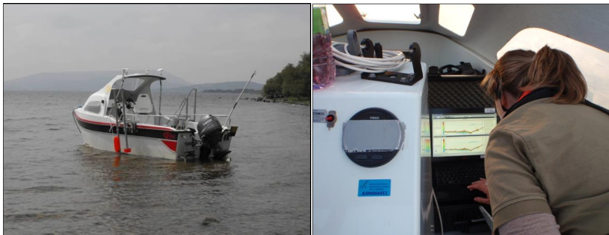
Plate 3.14. Left: Hydroacoustic transducers mounted on a boat (front - horizontally beaming, rear - vertical beaming). Transducers are lifted out of the water for illustrative purposes. Right: Laptop computer controlling the transducers via General Purpose Transceivers (GPT).
