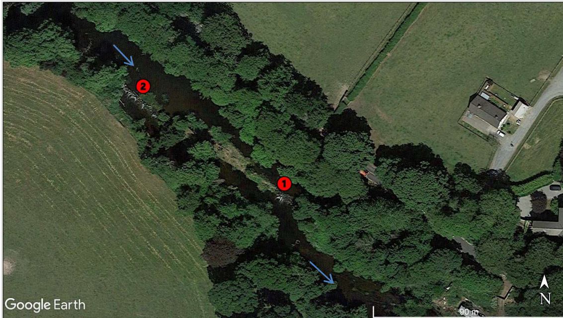
Figure 55. Google Earth ortho-image of Morristown Weir, June 2018. Blue arrows denote flow direction and red circles indicate transversal section number.
