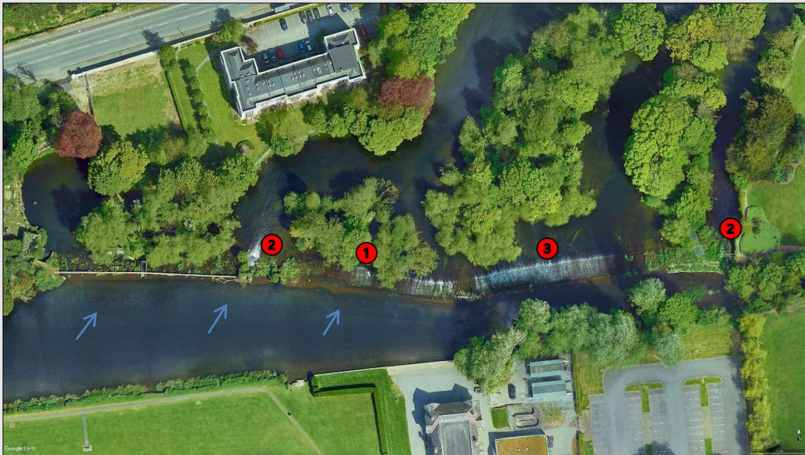
Figure 10. Google Earth ortho-imagery of Island Bridge Weir, April 2020. Blue arrows denote flow direction and red circles indicate transversal section number.
