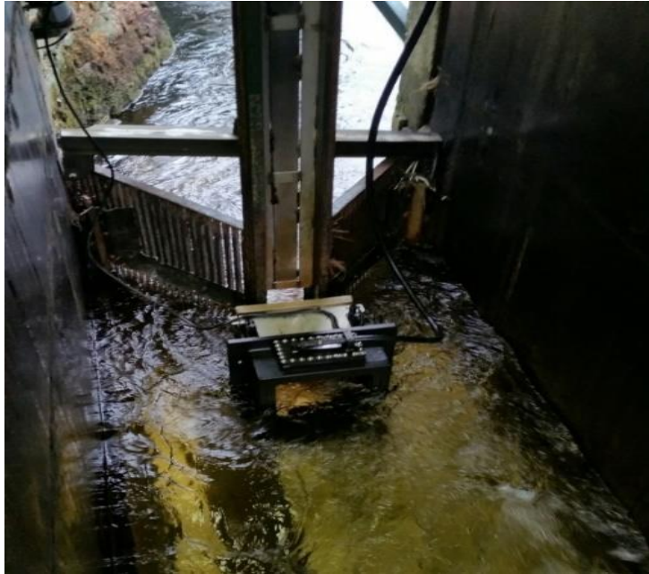
Figure 2 Erriff upstream trap with VAKI Riverwatcher counter and Biomark antenna (dark rectangular unit).
