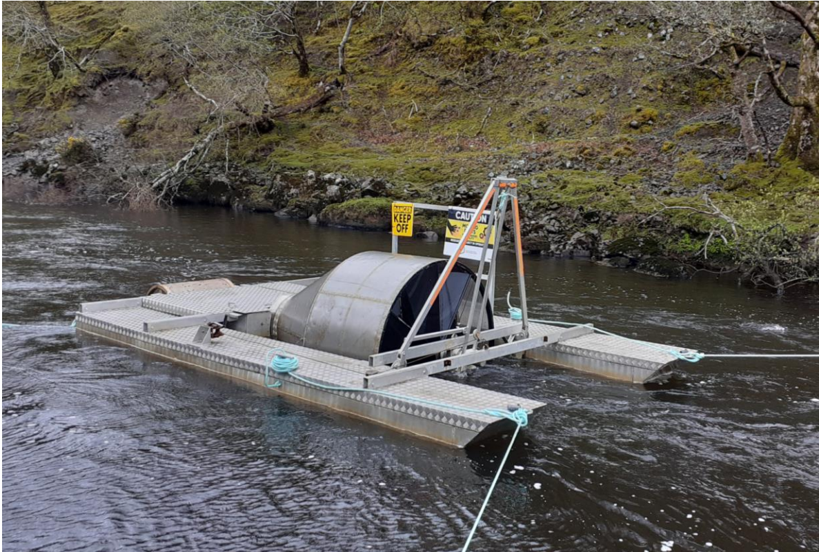
Figure 4 Rotary screw trap for capturing smolts in operation on the main river channel at Erriff Bridge.
