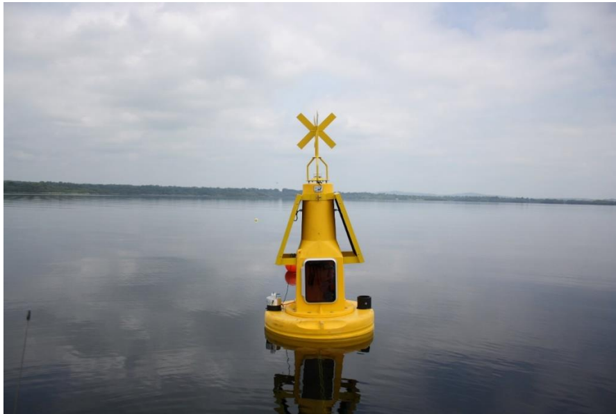
Figure 19. Lough Sheelin high frequency data buoy (monitoring water temperature (°C) throughout the water column (seven thermistors from surface) and water quality at the surface using a multiparameter water quality meter (e.g. dissolved oxygen, (% saturation and mg/l), conductivity ( \mu\text{S}/\text{cm} ) and chlorophyll a ).
