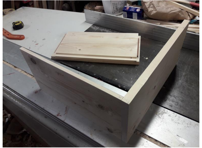
Side pieces being assembled for beehive
