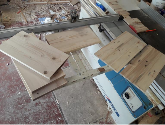
Wood cut to size to be used as sides for the brood box part of the beehive.
