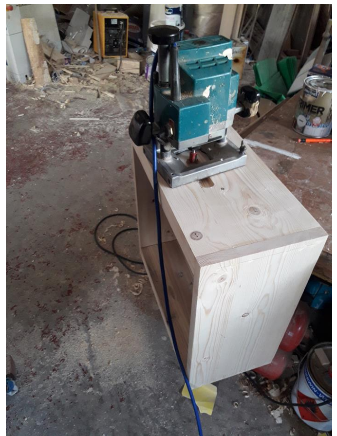
Router used to route handle pieces so the beehive can be easily carried.
