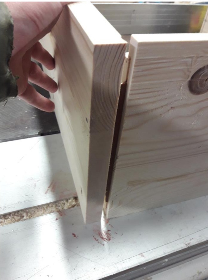
Biscuit joints used to join the side pieces to add strength to the structure of the beehive.
