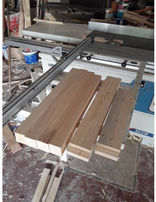
Wood cut and planed to size so it can be used as a stand.
