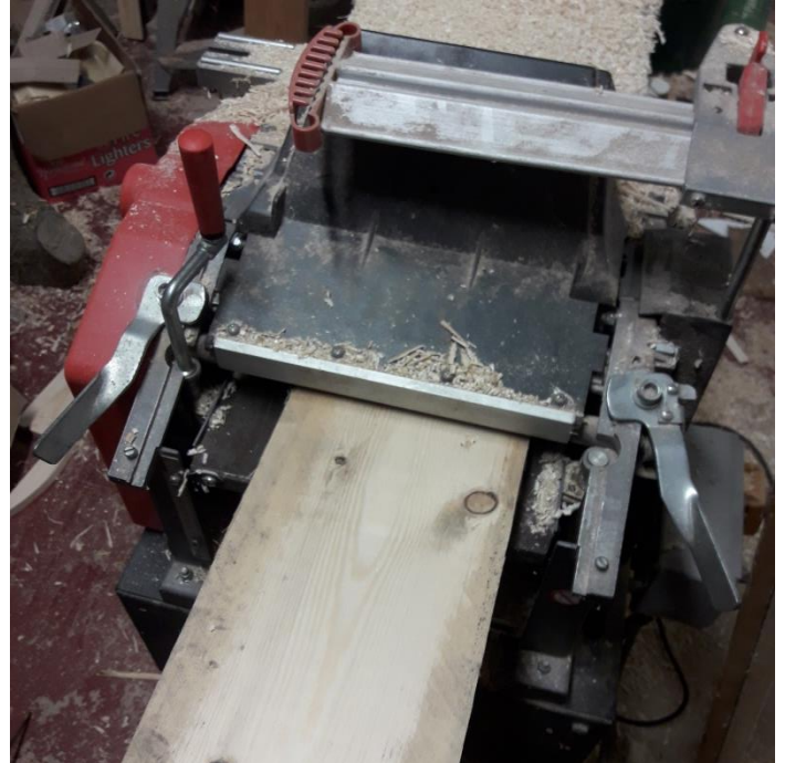
Pallet wood being planed to a suitable thickness
