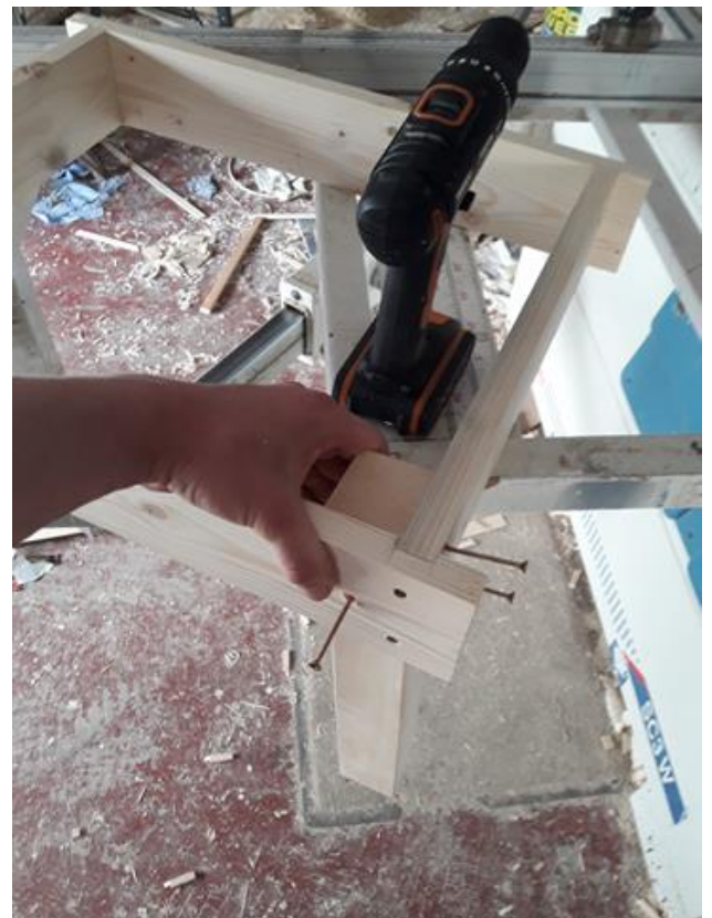
Assembly of stand using joints and screws.
