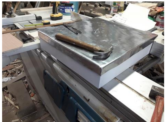
Aluminium sheet bent and attached to roof to prolong the life of the beehive.
