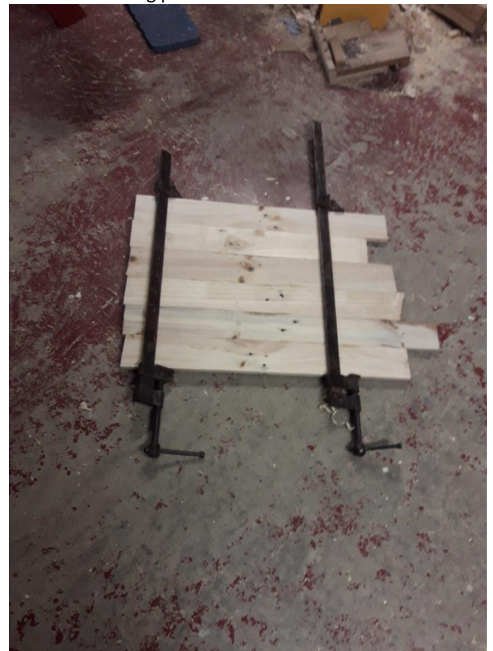
Gluing, joining and clamping of wood to be used for the floor of the beehive.
