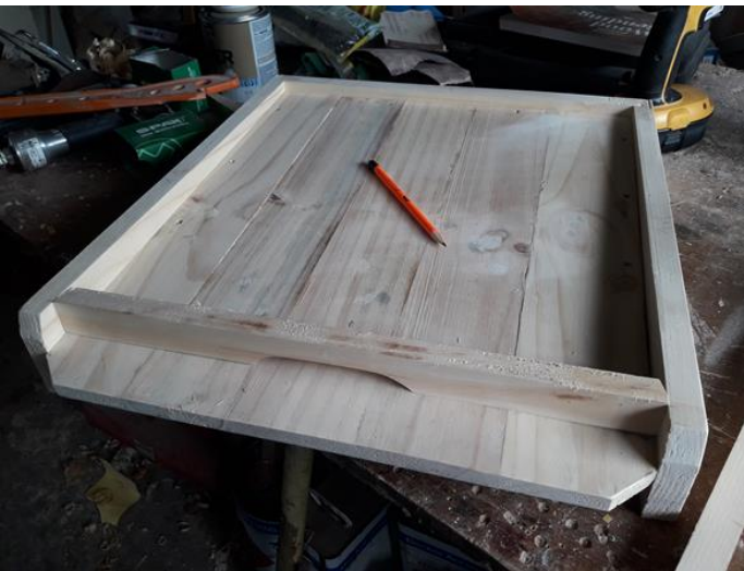
Finished beehive floor with entrance.
